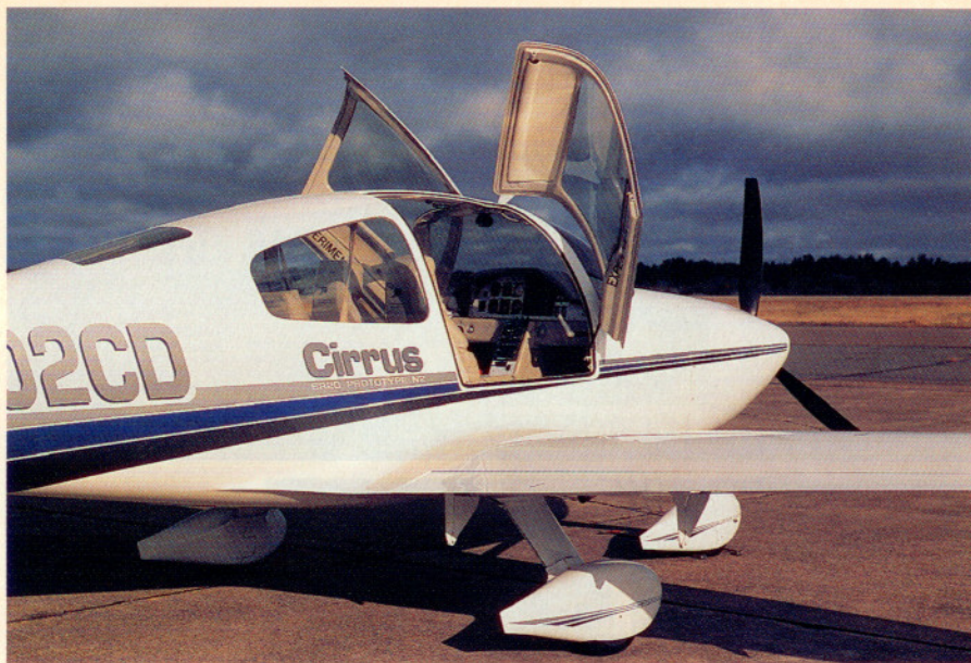
Gas struts hold the SR20's two cabin doors open in even the strongest gusts, while at the same time balancing the loads to make closing easy. The wide doors facilitate loading and unloading of the passenger compartment.
