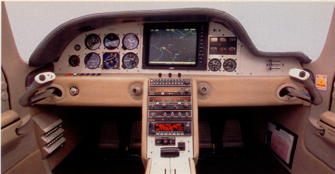
Cirrus SR20 prototype N2's panel arrangement is familiar and efficient (above). The production interior promises to be more car-like than that of the prototype airplane (left). Perhaps the most unusual feature of the interior is the sidestick controllers (below).
